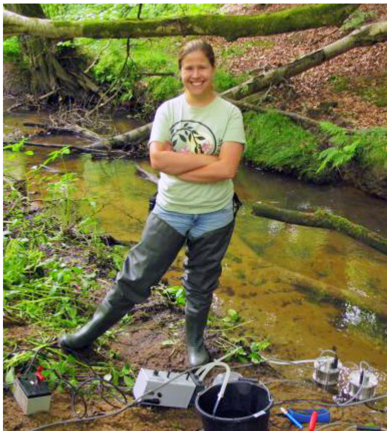
Marie Kurz calibrates fluorometers to measure tracer concentrations at a lowland stream in West Sussex, UK, in 2015. The data was later used by ORNL scientists to validate models of stream transport. Credit: Jay Zarnetske
