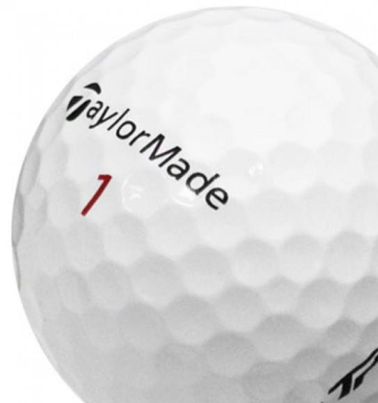
First, the dimples on the surface of a golf ball cause the boundary layer (outside) on the upstream side of the ball to transition from laminar to turbulent air flow. The turbulent boundary layer is able to remain attached to the surface of the ball much longer than a laminar boundary and so creates a narrower low-pressure wake and less pressure drag. The reduction in pressure drag causes the ball to travel further.
