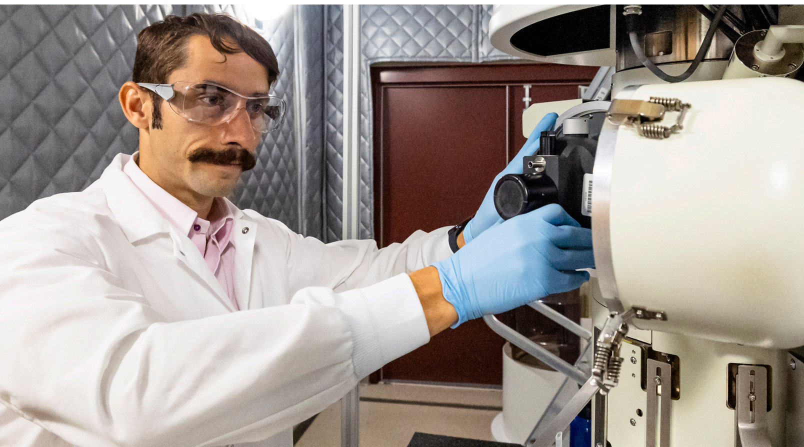
Fehmi Sami Yasin, an Associate R&D Scientist in ORNL's Scanning Transmission Electron Microscopy group, loads a liquid nitrogen cooled cryogenic side-entry holder to observe a metallic, ferromagnetic sample using transmission electron microscopy. Credit: Carlos Jones/ORNL, U.S. Dept. of Energy
