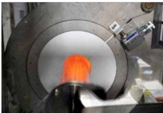
A stainless-steel disk was heated to create iron and nickel oxide particles on its surface. The particles catalyzed carbon nanotube growth during chemical vapor deposition. Credit: Carlos Jones/ORNL, U.S. Dept. of Energy
